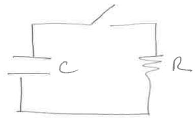
$$R = 1 \text{ M}\Omega \quad \left\{ \Rightarrow RC = 10^6 \times 10^{-6} = 1 \right.$$
