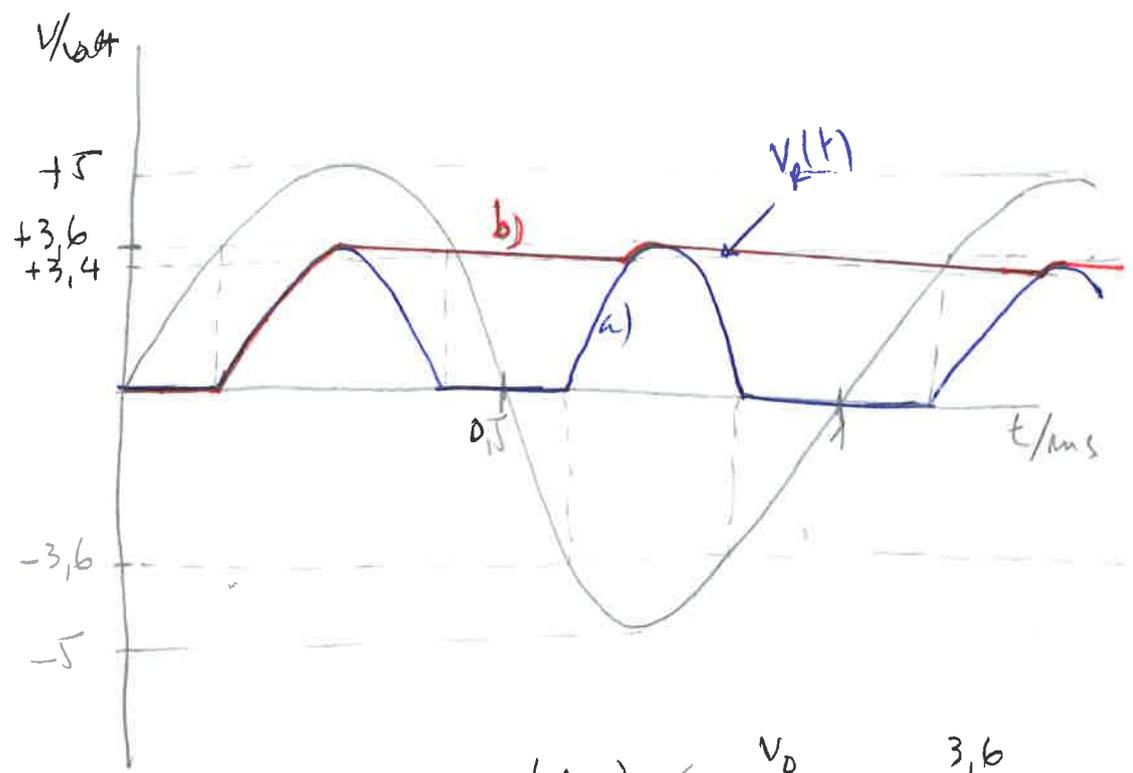
$(\Delta V_C)_{\text{máx}} < \frac{V_0}{2fRC} = \frac{3,6}{2 \times 10^3 \times 10^3 \times 10 \times 10^{-6}} \text{ V}$
